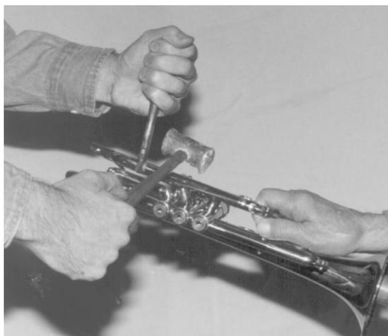
*When using slide pulling pliers, always inspect for braces that may bend or break from the stress of pulling. For example, on the cornet above, the casing to main slide brace is subject to damage. Have another person pull on the mouthpipe in opposition to the pulling force.*
