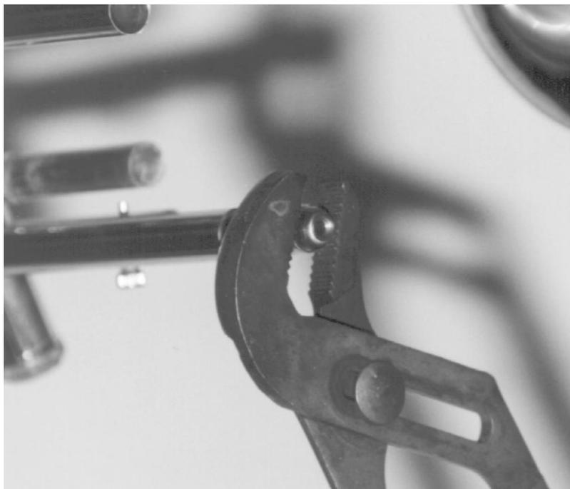
*If the ferrule is off the tube, some shops use slip-joint or channel lock pliers to grasp the tube directly, using barrel-shaped dent balls for support. While this will definitely mar the tube, the damage is limited to that area covered by the ferrule.*
