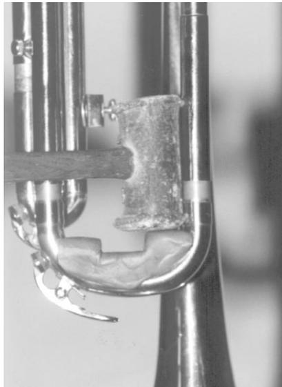
Epoxy Putty is a moldable compound that can be found at most hardware/home remodeling stores. It is easy to mix in one's hands and has a 20-minute working time. Grease acts as a release agent, preventing the putty from bonding to the part. Steel reinforced epoxy putties are available from machine tool suppliers.
