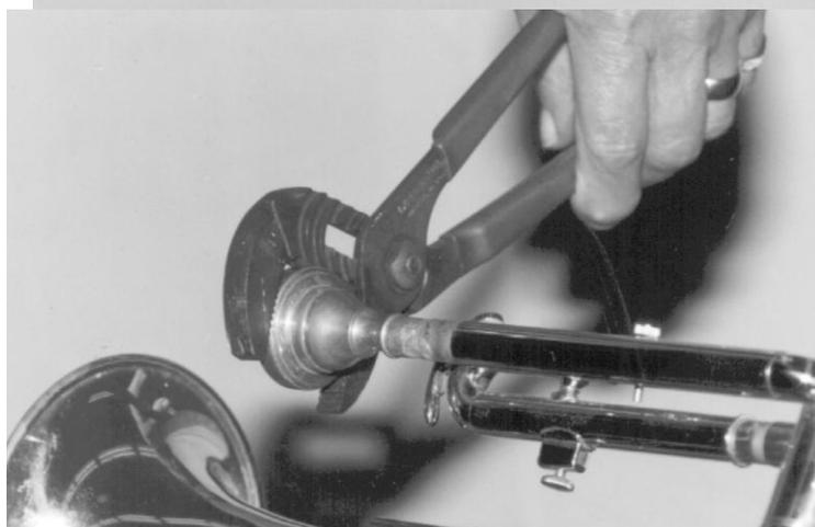
*On many brasswinds the crook can serve as a lever to pull the slide. Remove the crook and solder only one side back into the instrument. The tube can then be rotated out.*
